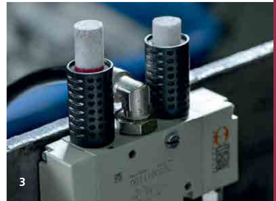
3. The warning mark indicates that the muffler needs replacing.
