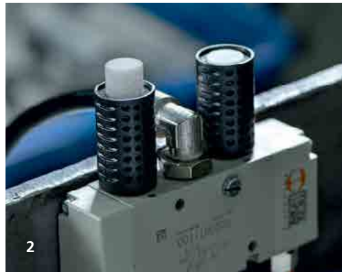
2. The muffler after a certain amount of clogging.
